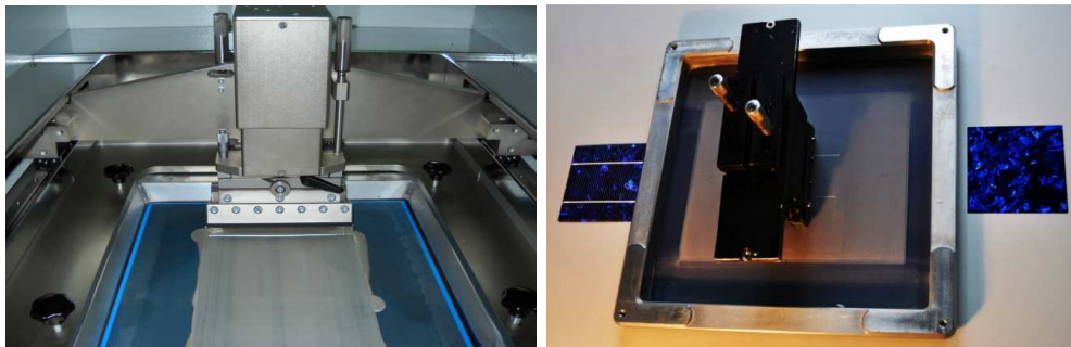
Fig. 20. System of squeegees brushing the paste over the sieve and pressing the paste through the meshes onto the plate's surface (left) and a sequence of paste printing in the process of creating the front electrode with the screen process method (right).
