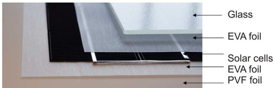
Fig. 38. Construction layers of a crystalline silicon-based photovoltaic module.
