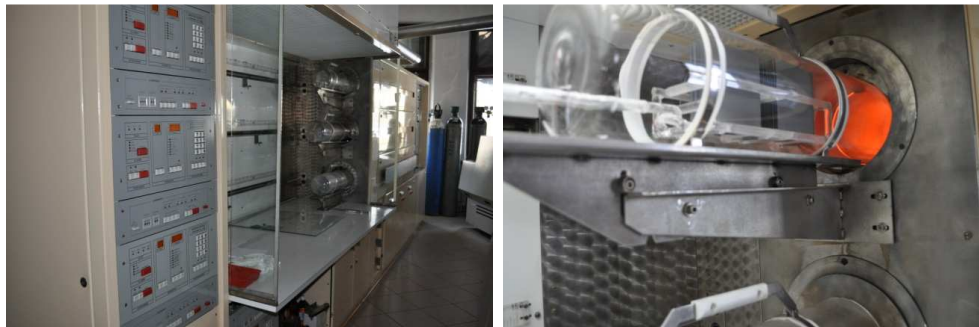
Fig. 14. Industrial diffusion furnace (left) the plate holder entering the heated quartz reactor (right)
