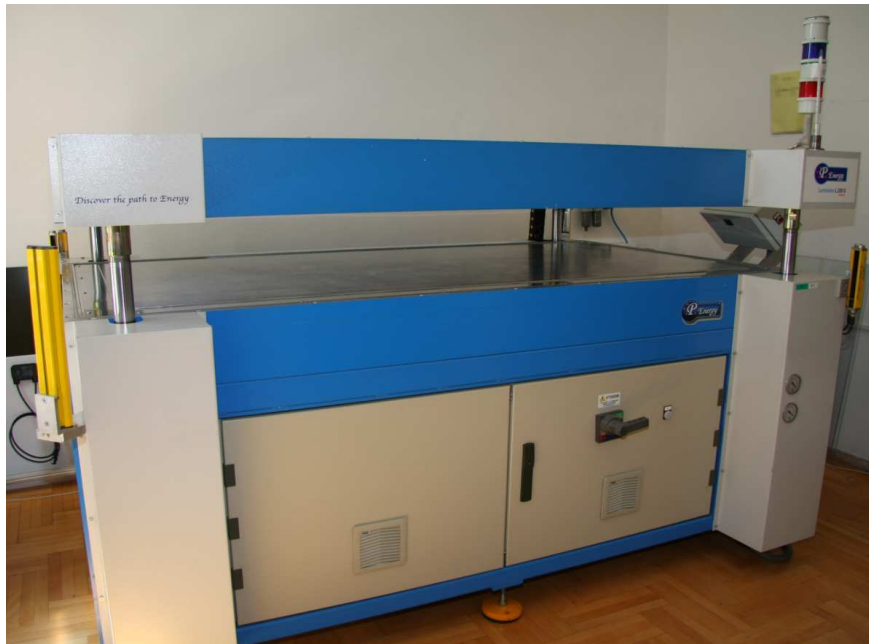
Fig. 39. Laminator L200, by the Italian producer Penergy, with an open lid of the heating chamber and a prepared system of layers for the lamination of a PV module, 50 cm wide and 100 cm long.
