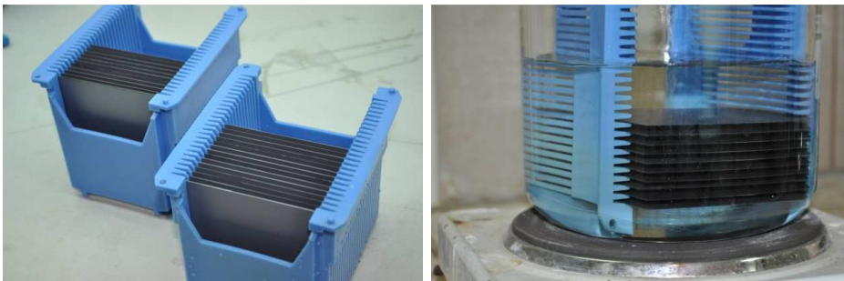
Fig. 12. Chemically prepared silicon wafers placed in teflon holders (left) and chemical etching process (right).
